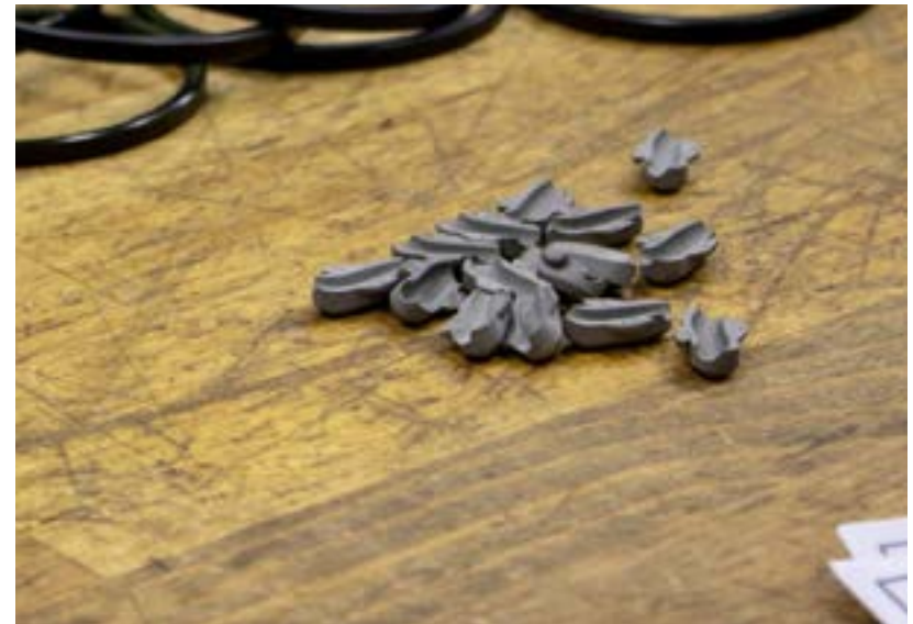
Printed converters are thus a suitable alternative for KSK Precise Motion compared to cast converters when dealing with non-standard or low-volume orders.
