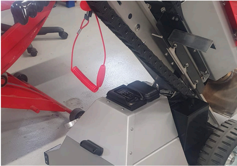
(Above: The final optimized battery case, painted black) Zirocco combines gas turbine technology with software to create effective surface drying equipment. Lightweighting Zirocco jet dryers improves product usability as they are operated manually.
