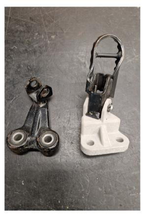
(Left) Orignal bracketinstalled.(Above) Orignal bracketcompared to extendedversion using 3Dprinted component.
