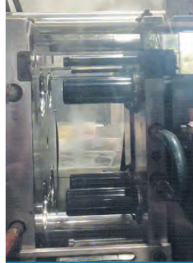
PRINTED INSERTS USED IN INJECTION MOLDING PRESS
